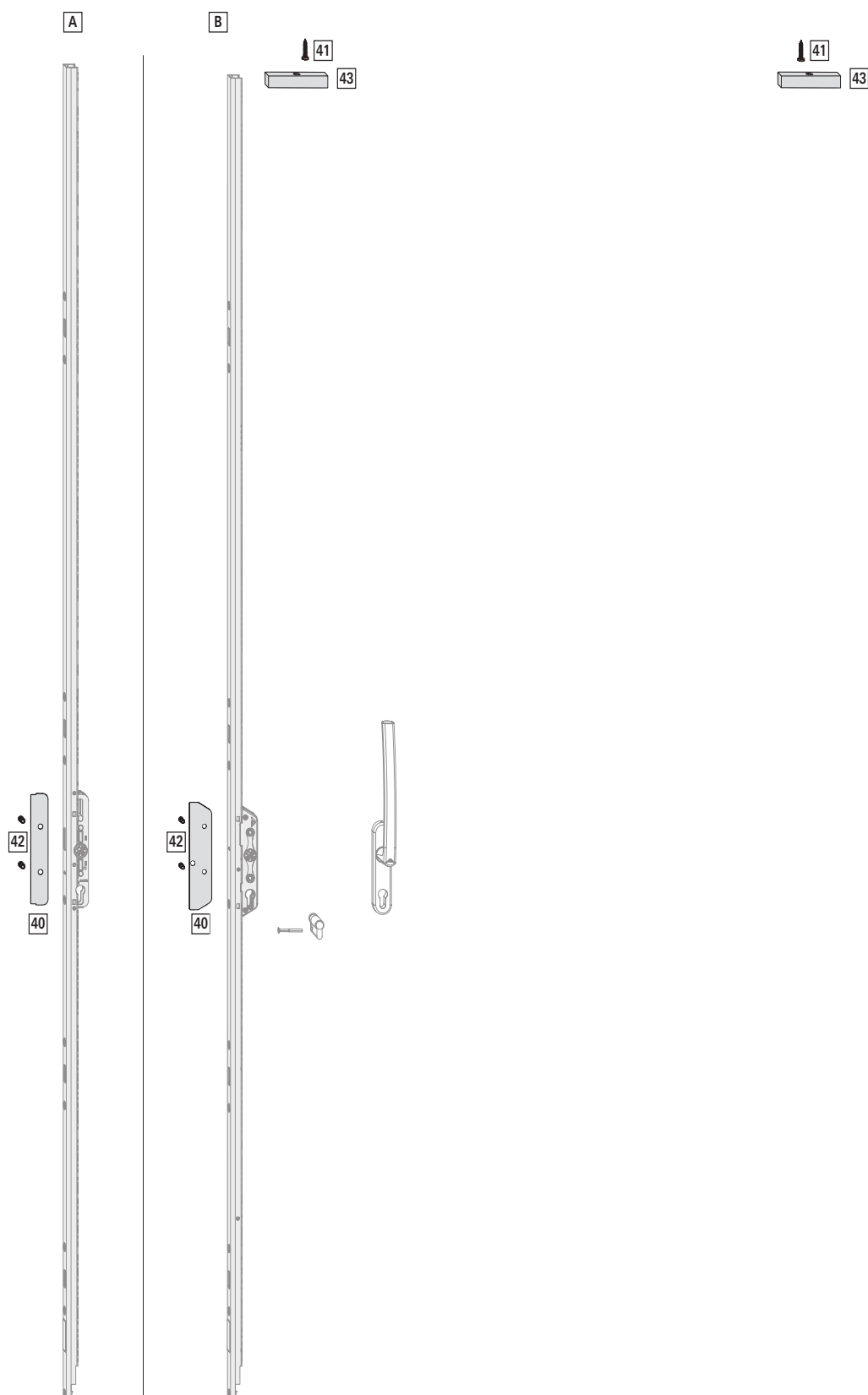
Fig. 4.11: Shown: diagram A; left version; SH 2400 mm; Slim [A] 200 kg and standard [B] S.kg 300 / 400 kg; lockable handles
